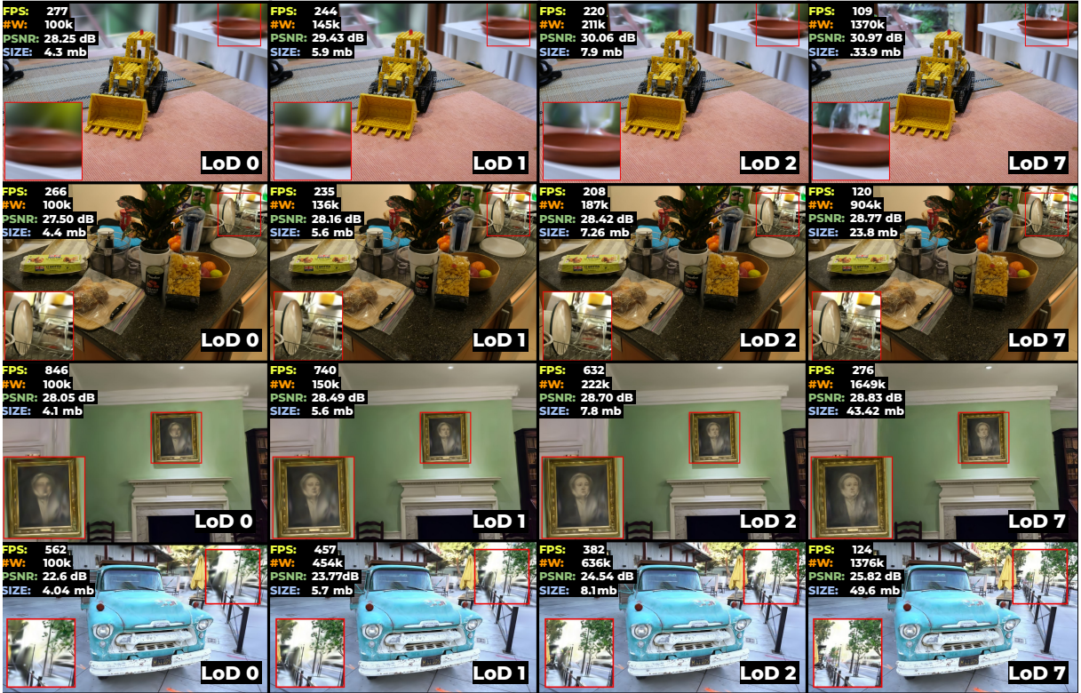
Fig. 4: Visualization of LoDs. For clarity, we show the first three levels and the final one. For each LoD, we report average FPS, PSNR, primitive count W (in thousands), and model size. From top to bottom: kitchen , counter , drjohnson , and truck .
